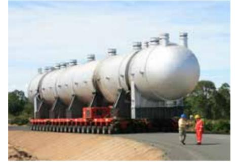
Figure 3: A titanium clad autoclave for nickel leaching. Image courtesy of COEK Engineering.
