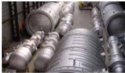
Figure 2: An array of titanium clad vessels and heat exchangers for a modern PTA plant. Image courtesy of COEK Engineering
