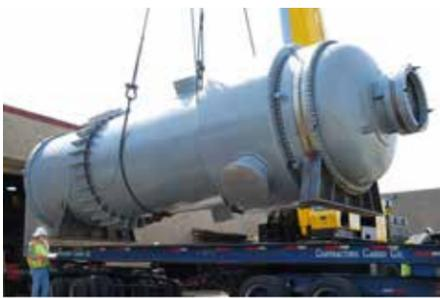
Figure 4: Shell and tube exchanger with titanium clad tubesheets for a high-pressure CPI application. Image courtesy of Titan Metal Fabricators
