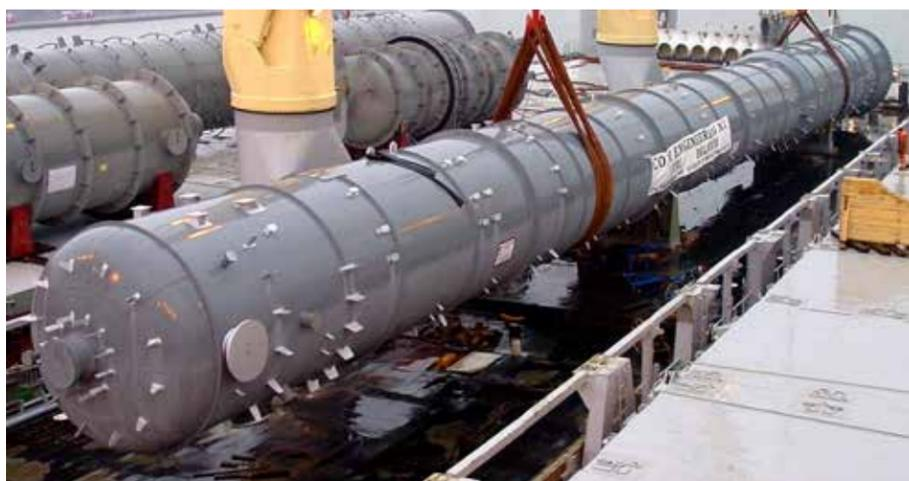
Figure 1: Titanium clad column for PTA. Image courtesy of COEK Engineering
