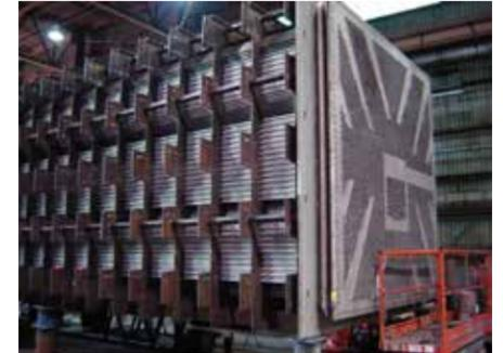
Figure 5: A condenser for a power generation plant, with 3 mm and 5 mm titanium clad tubesheets. Image courtesy of Holtec
