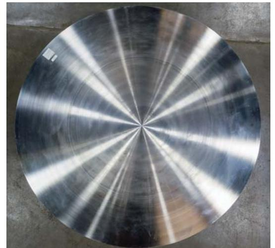
Fig. 2. An aerial view of a clad tubesheet inside the factory at NobelClad.
