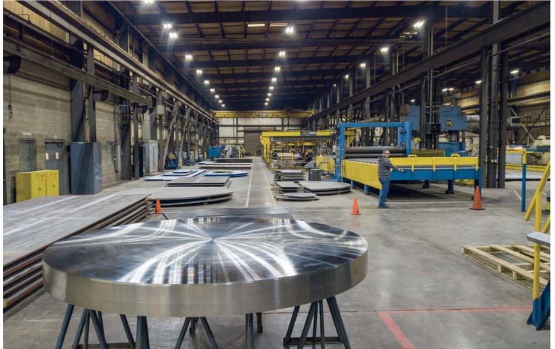
Fig. 1. A clad tubesheet prior to drilling.
