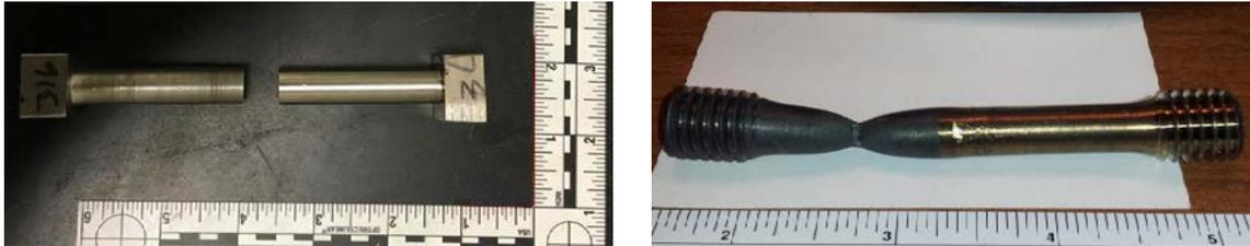
*Left: Roll bond clad that isn't qualified – brittle failure in the bondzone at room temperature.*
