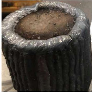
The sides of cylinders were cladded to prevent hydrogen from escaping. To accomplish this cladding, gas metal arc welding (GMAW), was employed to WOL the coupon blanks and put a top seal between the EXW and the sides as shown in Figure 4.
