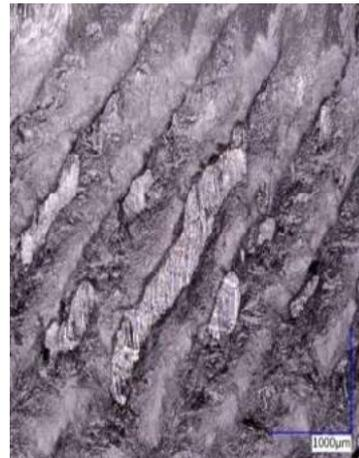
In the as-cladded condition (Figure 10), the interface showed a clear separation between the Bainite structure of the steel and the austenitic structure of AISI 321 cladder. There was no evidence of martensitic structure potentially detrimental for such applications.
