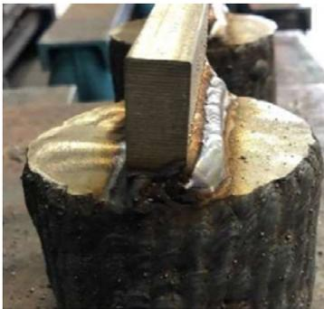
**Figure 5:** ASTM G146 Specimen for DirectAttach™
