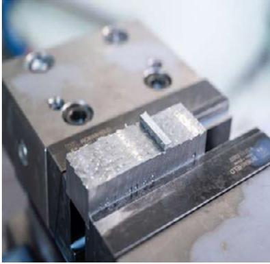
**Figure 7:** Shear test according to ASME SA-264
