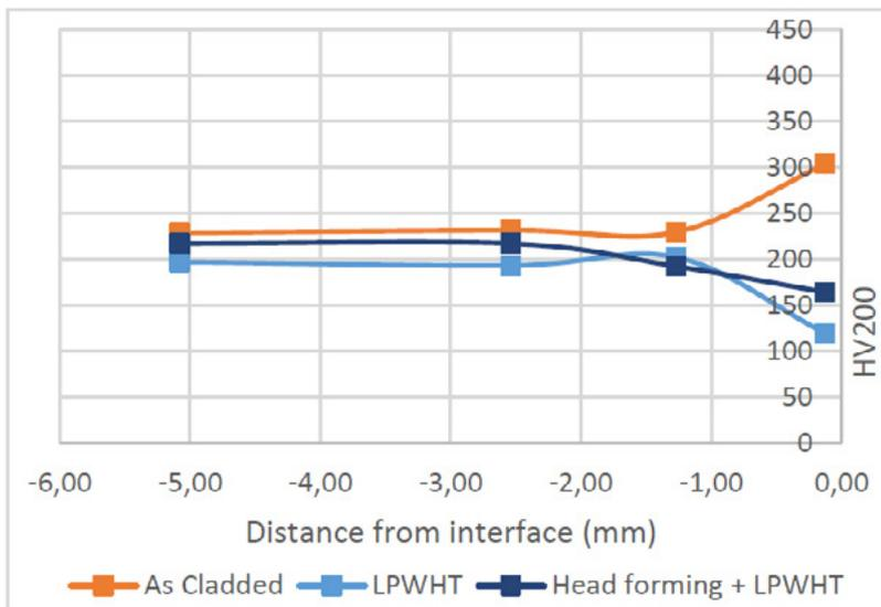
**Figure 12:** Microhardness data on steel from EXW interface
