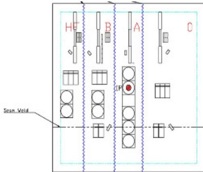
Figure 2: Testing specimen layout incorporating variety of DetaClad™ configurations.
